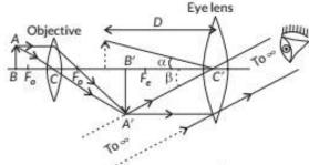
Magnification due to objective,  $m_0 = \frac{L}{-L}$
