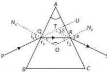
At the face AB, the angle of incidence is  $i_1$  and angle of refraction is  $r_1$ . So the deviation at this surface is
