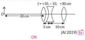
Three lenses of focal lengths +10 cm, -10 cm and +30 cm are arranged coaxially as in the figure given
