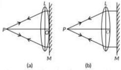
From figure, focal length of lens = OP = 20 cm
