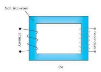
The working principle of transformer is mutual induction.
