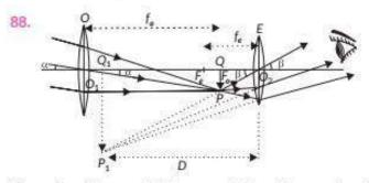
Here,  $f_o$  = 15 m = 1500 cm and  $f_e$  = 1.0 cm. Angular magnification by the telescope in normal adjustment
