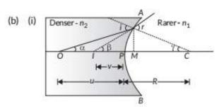
Relationship between the object distance and image distance in terms of n<sub>1</sub>, n<sub>2</sub> and R for a concave spherical surface.
