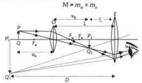
When the final image is formed at infinity (normal adjustment).
