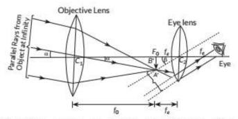
Magnifying power or angular magnification of an astronomical telescope in normal adjustment is defined as the ratio of the angle subtended at the eye by the final image to the angle subtended at the eye by the object directly, when the final image and the object, both at infinite distance from the eye.
