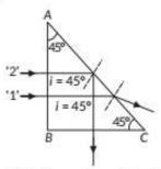
Both the rays will fall on the side AC with angle of incidence, i equal to 45°. Critical angle of ray '1' is greater than i. Hence, it will emerge from the prism as shown in the figure.
