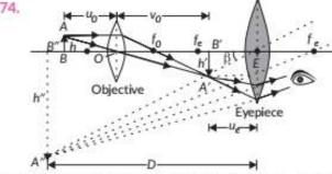
Compound microscope consists of two convergent lenses of short focal lengths and apertures arranged co-axially. Lens (of focal length  $f_o$ ) facing the object is known as objective or field lens while the lens (of focal length  $f_e$ ) facing the eye, is known as eye-piece or ocular. The objective has a smaller aperture and smaller focal length than eye-piece. Magnifying power of a compound microscope
