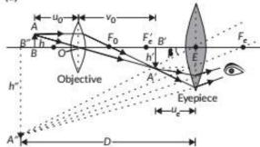
(b) Separation between eye-piece and the objective,  $L = 14 \text{ cm}, m = -20, m_e = 5, D = 20 \text{ cm}, f_o = ?, f_e = ?$ Magnification of eye-piece when image is formed at the least distance for clear vision.
