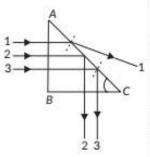
65. (i) Optical fibre is made up of very fine quality glass or quartz of refractive index about 1.7. A light beam incident on one end of an optical fibre at appropriate angle refracts into the fibre and undergoes repeated total internal reflections.
