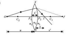
For refraction at spherical surface  $XP_1Y$ , object is at O and image is at I'.
