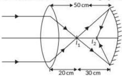
The image  $I_1$  is formed in front of the mirror and hence, acts as a real source for the mirror. The concave mirror forms the image  $l_2$ . For the concave mirror, u = -30 cm and f = -10 cm
