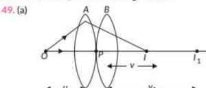
An object is placed at point O. The lens A produces an image at I1 which serves as a virtual object for lens B which produces final image at I.
