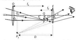
Ray diagram of astronomical telescope when final image is formed at infinity.
