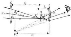
Magnifying power of refracting telescope (M) is defined as the ratio of the angle subtended by the image ( $\beta$ ) at the eye to the angle subtended by the distant object at the unaided eye ( $\alpha$ ).
